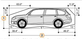
Vehicle width of 74.9" with a platform width of 90.6". Wider platforms allow correspondingly wider vehicles to be parked.
