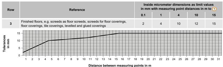
1 Intermediate values must be taken from the diagram and rounded up.
