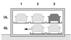
To remove the vehicle from the space in **grid 3/UL**, the GL platforms are moved to the left
