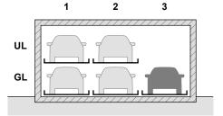
The vehicle in the space in **grid 3/UL** can now be removed.
