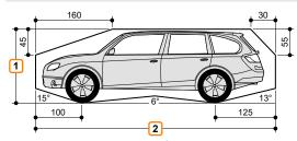
Vehicle width 190 cm with platform width 230 cm. Correspondingly wider vehicles can be parked with wider platforms.
