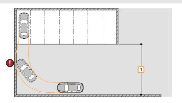
All side walls must be at a right angle. Maximum deviation 1 cm!
