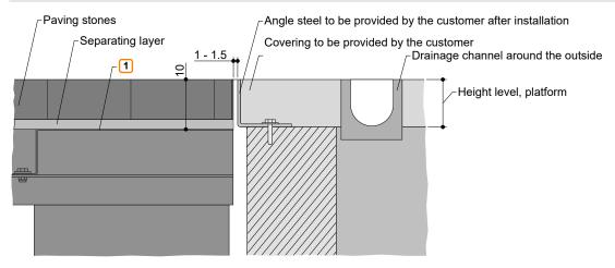
1 Sealing of the pit (see "Detail of building configuration - pit sealing", page 8)
