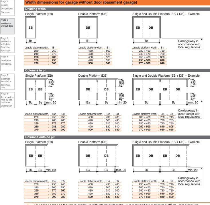
For parking boxes on the edges and boxes with intermediate walls we recommend our maximum platform width of 270 cm for single platforms and 500 for double platforms. Problems may occur if smaller platform widths are used (depending on car type, access and individual driving behaviour and capability).
