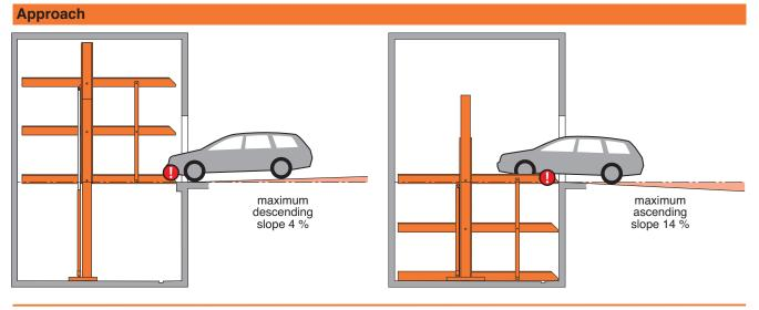
The illustrated maximum approach angles must not be exceeded. Incorrect approach angles will cause serious maneouvring & positioning problems on the parking system for which the local agency of KLAUS Multiparking accepts no responsibility.
