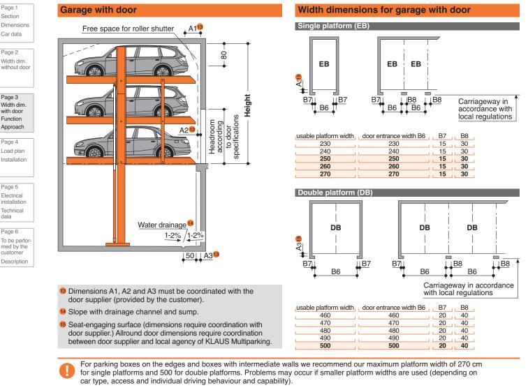
For larger limousines and SUV wider driveways are necessary (in particular on the boxes on the sides due to the missing manoeuvring radius).
