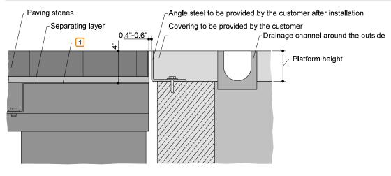
1 Trough seal (see "Detail of building design – trough seal", page 8)
