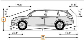
Vehicle width of 74.9" with a platform width of 90.6". Wider platforms allow correspondingly wider vehicles to be parked.
