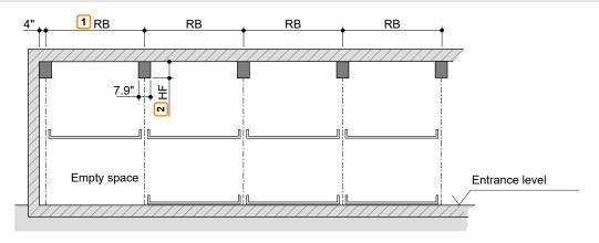
1 RB: grid width. This dimension **must** be adhered to!
