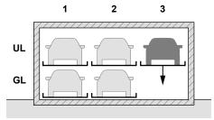
The empty space is now located under the vehicle being removed. The parking space in **grid 3/UL** is lowered.
