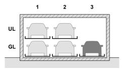
The vehicle in the space in **grid 3/UL** can now be removed.
